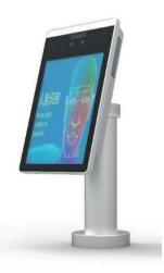
Face reader access control terminal integrates certificate ID, facial recognition with TCP/IP communication.All terminals can be managed by internet to control lock and realized data backup.
