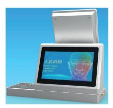
Face reader access control terminal integrates certificate ID, facial recognition with TCP/IP communication.All terminals can be managed by internet to control lock and realized data backup.
