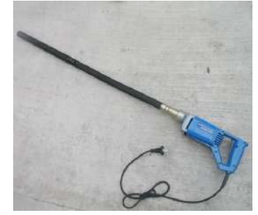
Concrete Vibrator Shaft
