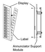
the 3-LCDXL1 has a larger 240 x 320 pixel backlit display that supports 24 lines of 40 characters. Both LDC displays provide the room needed to convey emergency information in a useful format.
