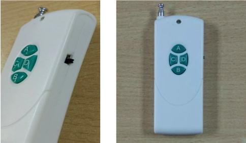
Switch is on the side of remote control. Total four buttons on remote controller. A(Up), B(Down), C(Stop), D(Spare Key).
