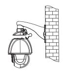
6 Fix the bracket to the wall with the screws and then hook the safety wire to the tub.
